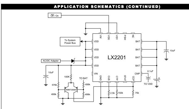
Figure 7 – AC Adapter with charging voltage headroom regulation (for use with a current limited power supply).
