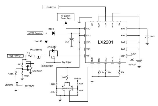
Figure 8 - Current limited USB interface with isolated battery and bi-directional pass element.
